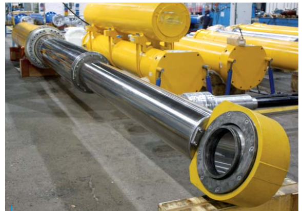
BOP Elevator Telescopic Cylinder 650 x 570, 480 x 380, Stroke 6 100 mm with METALTEK® rod coating
